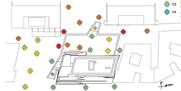
FIGURE 14b SUMMARY OF PREDICTED COMFORT LEVELS FOR PEDESTRIAN-LEVEL WIND SPEEDS
